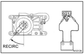
(2) Connect the positive (+) lead from the battery to terminal 1 and the negative (-) lead to terminal 2, check that the arm rotates to the "RECIRC" side smoothly,
