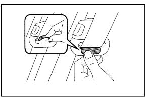
D. Remove the lower side colored film from the fluorocarbon resin tape, and securely affix the tape to the outside of the shoulder belt anchor.
