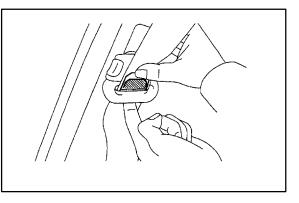
C. Remove the upper side colored film from the fluorocarbon resin tape, and securely affix the tape to the outside of the shoulder belt anchor.
