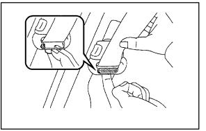
Installation Procedure (Continued) F. By pulling the seat belt up and down several times, as shown in the illustration, securely affix the fluorocarbon resin tape and confirm the smoothness of the belt movement.
