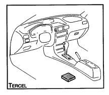
1. '98 Model and prior has ECU located beneath the driver's seat.
