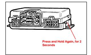
4. Turn off the ignition. The ECU has cleared all REMOTE CONTROL codes; until another REMOTE CONTROL is programmed, the system will not work with any REMOTE CONTROL.
