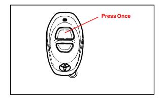
\* Either button on your REMOTE CONTROL can be programmed to operate the system. The bottom button can be programmed to operate a second vehicle with the Toyota VIP.
