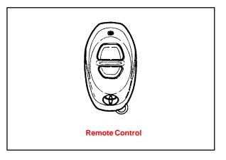
The DIO or PIO Keyless Entry System utilizes only remote controls with **black** cases. The same remote controls but with **gray** cases, used for 1998 MY and later RS3000 TVIP systems, will not work with this keyless entry system.
