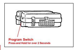
Press and hold the ECU's PROGRAMMING SWITCH for over 2 seconds again.
