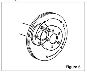
Tighten lug nuts to the specified torque following a star sequence when installing wheel
