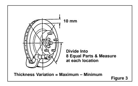
There are two factors which cause excessive rotor thickness variation:
