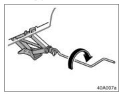
5. After making sure that no one is in the vehicle, raise it high enough so that the spare tire can be installed.
