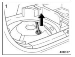
1. Remove the towing eyelet as shown in the illustration.
