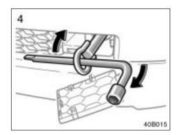
4. Tighten the towing eyelet securely by a wheel nut wrench.
