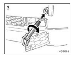
3. Secure the towing eyelet to the hole on the bumper by turning clockwise.
