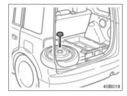
To remove the spare tire, loosen the bolt and remove it.
