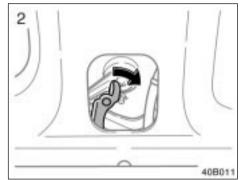
2. Push the lever with the back door motor, open the back door.
