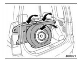
Put the flat tire on the center of the luggage floor. Then hold the deck boards (with the front side facing toward the back of the vehicle) between the rear seatback and flat tire.
