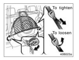
Hook the 2 hooks and adjust the belt so that the strap does not allow the slack.
