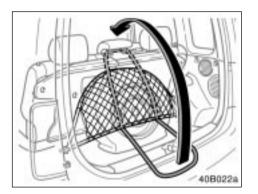
Wrap the flat tire with the flat tire net and hook the strap on the rear center head restraint.
