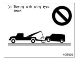
(c) Towing with sling type truck
