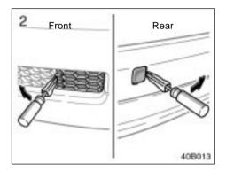
2. Remove the towing eyelet cover on the bumper using a flathead screwdriver which is wrapped with a cloth.
