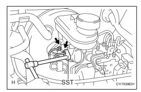
(c) Install the brake master cylinder reservoir with the reservoir stopper.
