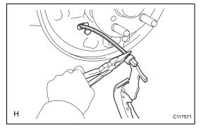
(b) Using needle-nose pliers, disconnect the No. 3 parking brake cable from the parking brake shoe lever.
