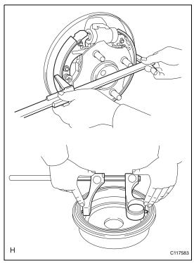
(b) Measure the inside diameter of the brake drum and diameter of the brake shoe. Check that the difference between the diameters is the correct shoe clearance.
