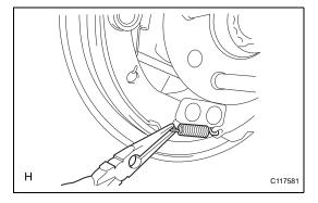
(c) Using needle-nose pliers, connect the tension spring to the front brake shoe and rear brake shoe.
