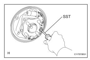
(b) Using SST, install the rear brake shoe, pin, shoe hold down spring and shoe hold down spring cup.SST 09718-00010
