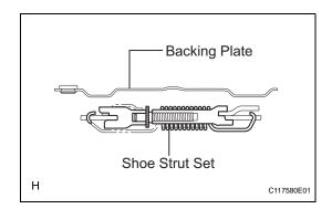
(c) Install the shoe strut as shown in the illustration.
