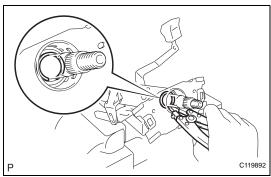
(c) Using a snap ring expander, install a new snap ring to the upper side.
