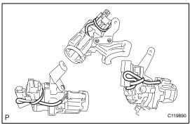
(c) Using a new clamp, fix the wire harness of the unlock warning switch to the steering column bracket upper as shown in the illustration.
