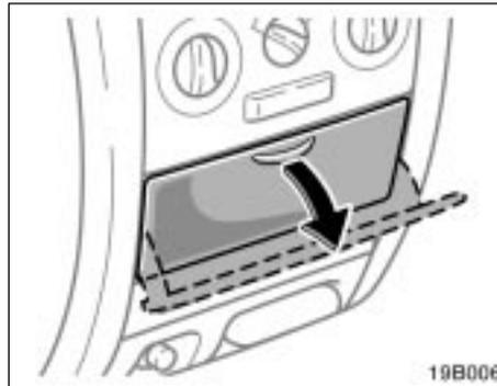
To use the box, pull on the handle. You can find the card holder on the back side of the box lid.
