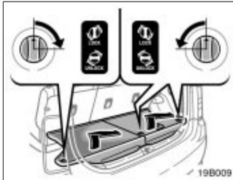
To open the luggage storage box, turn the knobs to the “UNLOCK” position and open the lid. To close the luggage storage box, lower the lid and turn the knobs to the “LOCK” position.
