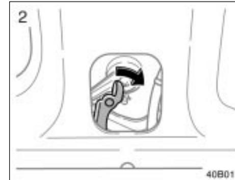
2. Push the lever with the back door motor, open the back door.
