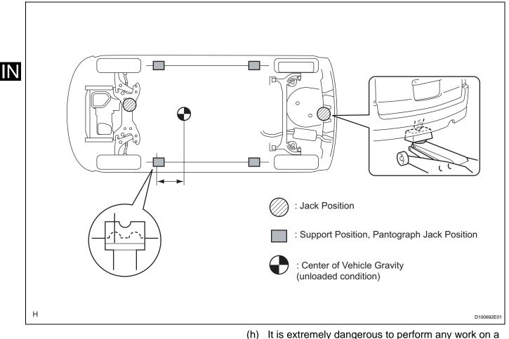
(h) It is extremely dangerous to perform any work on a vehicle raised on a jack alone, even for work that can be finished quickly. Safety stands must be used to support it.
