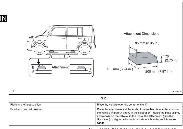
(d) Use the lift to raise the vehicle up off the ground, and shake it to make sure that it is stable.
