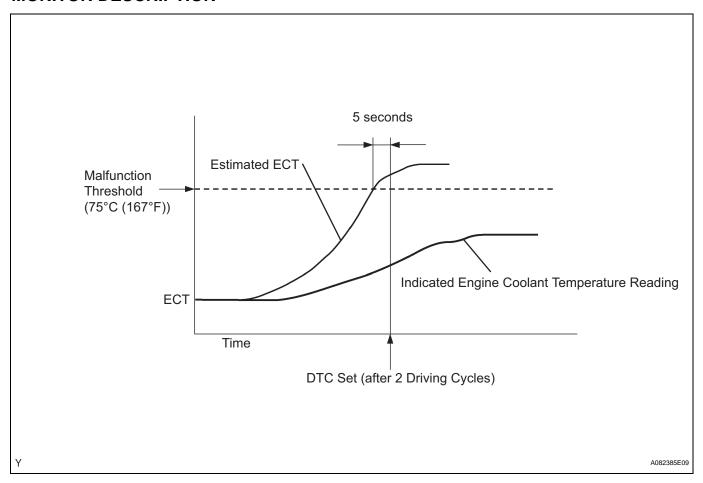
The ECM estimates the ECT based on starting temperature, engine loads, and engine speeds. The ECM then compares the estimated temperature with the actual ECT. When the estimated ECT reaches 75°C (167°F), the ECM checks the actual ECT. If the actual ECT is less than 75°C (167°F), the ECM will interpret this as a malfunction in the thermostat or the engine cooling system and sets the DTC.
