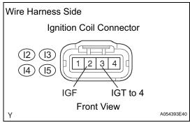
(c) Measure the resistance of the wire harness side connectors.
