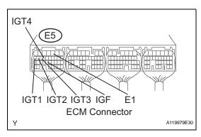
(a) Inspect the ECM using an oscilloscope.
