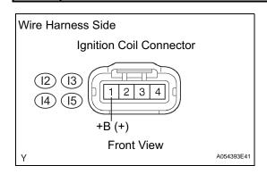
(a) Disconnect the I2, I3, I4 or I5 ignition coil connector.
