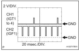
(b) While cranking or idling, check the waveform between the terminals of the E5 ECM connectors.
