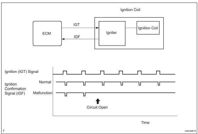
If the ECM does not receive any IGF1 signals despite transmitting the IGT signal, it interprets this as a fault in the igniter and sets a DTC.
