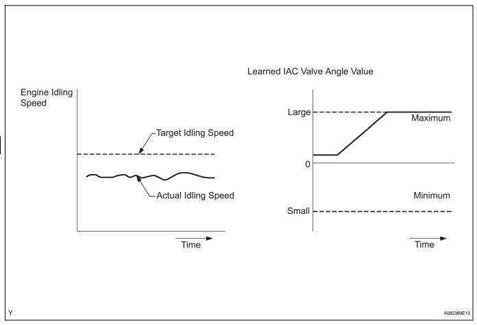
The IAC valve controls the volume of air that bypasses the throttle valve.
