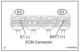
(a) Measure the voltage of the E3 and E5 ECM connectors. **Standard voltage**
