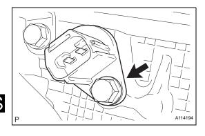
(b) Connect the sensor connector.
