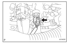
(b) Remove the sensor and gasket.
