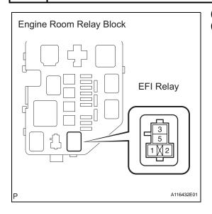
(a) Remove the EFI relay from the engine room relay block.(b) Disconnect the M1 MAF meter connector.
