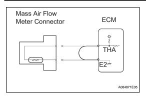
(a) Disconnect the M1 MAF meter connector.
