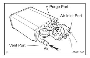
(2) While holding the air inlet port closed, blow air 0.39 kPa (4.0 kgf/cm<sup>2</sup>, 3 mmHg) into the vent port, and check that air flows from the purge port.
