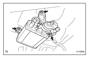
(c) Remove the 3 bolts and canister.
