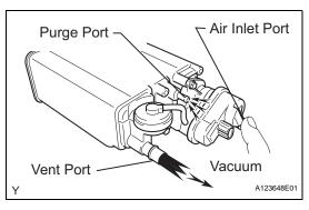
(3) While holding the air inlet port closed, apply vacuum 3.43 kPa (35.0 kgf/cm<sup>2</sup>, 25.7 mmHg) to the vent port, and check that air is sucked into the purge port.
