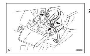
(c) Connect the connector and attach the 2 clamps.
