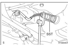
(b) Using SST, remove the sensor. **SST 09224-00010**
