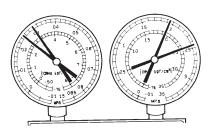
HINT: These gauge indications occur when the refrigeration system opens and the refrigerant is charged without vacuum purging
