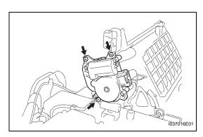
(c) Detach the 2 clamps and disconnect the wire harness.
