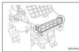
8. INSTALL DAMPER SERVO SUB-ASSEMBLY(a) Install the damper servo with the 3 screws.
