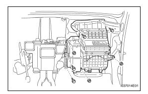
(b) Install the A/C blower with the 4 bolts and 3 nuts.
