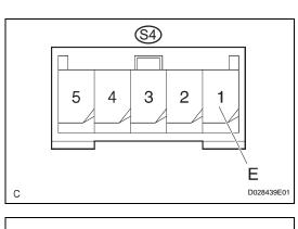
Connector A: Shift Lock Control Switch Side
