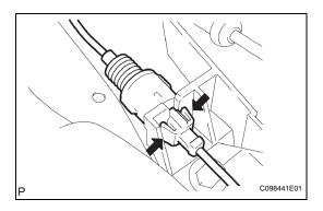
(c) Using a screwdriver, disconnect the floor shift parking lock cable from the shift lever plate.
