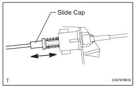
(h) Hold the slide cap and move it back and forth. Check that the spring for automatic adjustment works properly.
