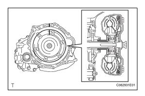
(d) Align the marks on the case and converter clutch, and fit the splined part of the input shaft to the spline part of the turbine runner.
