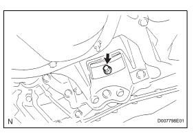
(b) Install the 6 torque converter mounting bolts.
