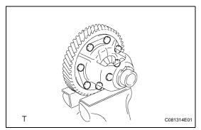
(c) Remove the 8 bolts and lock plate.
