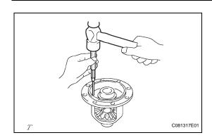
(b) Using a pin punch and hammer, tap out the straight pin.
