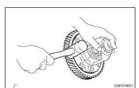
(d) Using a plastic-faced hammer, tap out the front differential ring gear from the differential case.
