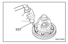
(b) Using SST and a hammer, unstake the lock plate. **SST 09930-00010**
