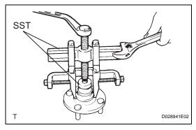
(b) Using SST, remove the inner race of the hub bearing from the axle hub.
