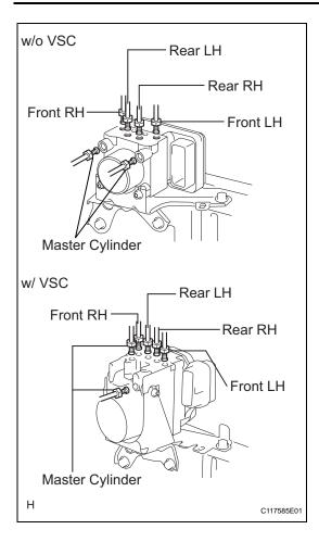
(c) Place tags or marks to identify the installation locations of each brake line.
