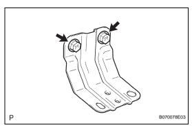
(c) Install the bracket with the 2 screws.
