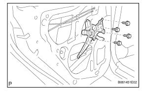
(i) Connect the No. 2 remote control rod in the direction indicated by the arrow marks in the illustration.
