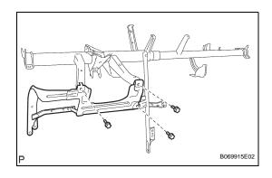
(b) Install the instrument panel lower pad insert LH with the 3 bolts.
