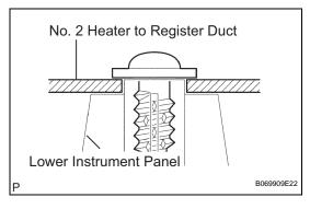
(b) Using a screw, install the No. 2 heater to register duct.
