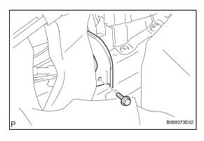
(j) Install the No. 1 instrument panel mounting bracket with the bolt.
