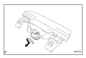
(c) Remove the stop light bulb as shown in the illustration.
