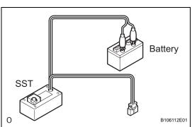
(1) Connect the SST's red clip to the battery's positive (+) terminal and the black clip to the battery's negative (-) terminal.
