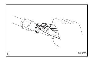
(c) Using a snap ring expander, remove the snap ring on the lower side.
