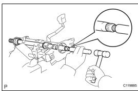
(b) Using an extension bar and hammer, tap out the steering main shaft.
