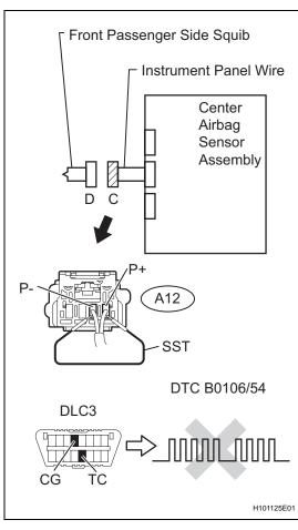
(b) Using SST, connect terminals P+ and P- of connector "C".
