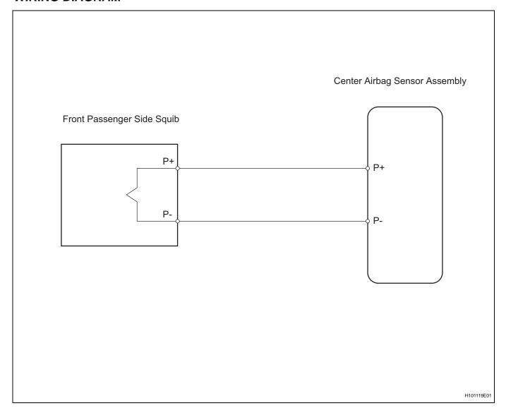
1 CHECK INSTRUMENT PANEL WIRE (FRONT PASSENGER SIDE SQUIB CIRCUIT)
