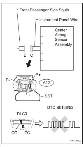
(d) Using SST, connect the terminals P+ and P- of connector "C".
