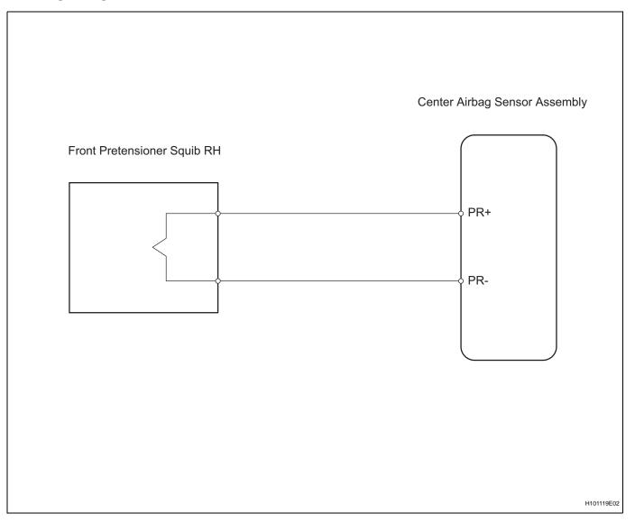
1 CHECK FLOOR WIRE (FRONT PRETENSIONER SQUIB RH CIRCUIT)
