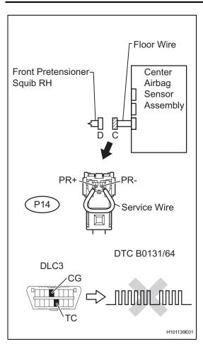
(b) Using a service wire, connect terminals PR+ and PR- of connector "C".
