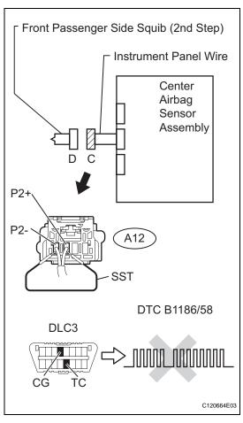
(b) Using SST, connect terminals P2+ and P2- of connector "C".
