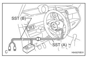
(1) Connect the SST's red clip to the positive (+) battery terminal and the black clip to the negative (-) battery terminal. HINT:
