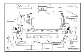
(a) Attach the 12 claws to install the front passenger airbag.
