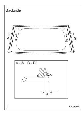
(b) Install a new moulding LH and RH as shown in the illustration.
