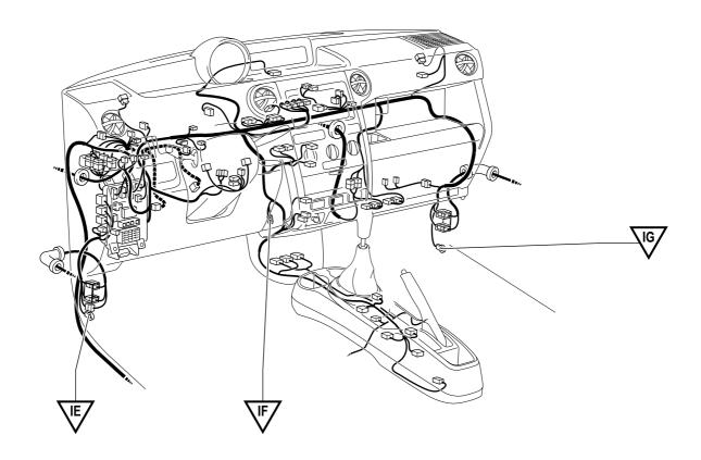
☐ : Location of Connector Joining Wire Harness and Wire Harness
