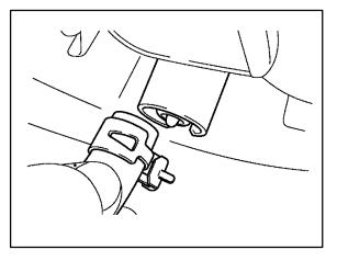
3. Push the drain hose up onto the evaporator drain tube. Ensure that the drain hose is up far enough for the retaining clamp to fully engage the tube.
