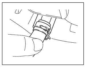
**Repair** 4. Release the holding clip. **Procedure** (Continued)
