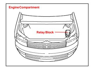
During Pre-Delivery Service (PDS), install the DOME fuse (15A) in the Relay Block as shown.
